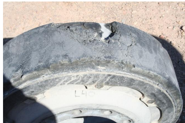
Figure 8: Example of a nearly failed road wheel; "failure" of a road wheel defined as 50% rubber lost
